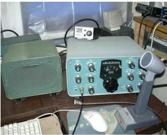
A restored Heathkit SB-102 transceiver, 100 watts on 80 thru 10 meters. Shown with the Heathkit SB-600 Speaker which contains an Hp-23A high voltage power supply. The microphone is a Shure model 444D.
